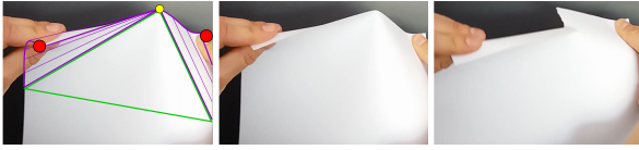
Figure 5: Junction points (yellow point) in this real case scenario are specific points on the papers boundary from which a tearing path is supposed to start.
