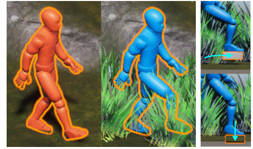
Figure 3: We use a moving platform (right) acting as a fake target ground for the foot, but suddenly moving down when hit, to model the presence of grass and its ability to be crushed.
