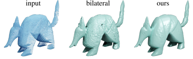
Figure 3: When normals are missing: Approaches such as bilateral filtering require normal estimates along with the input pointset; deducing normals from a local neighborhood PCA or more advanced normal estimators [CCC*08] results in bumpy surfaces (left), while our variational approach manages to denoise the input reliably without normal guesses (right). The scanned Armadillo model is from [HWG*13].
